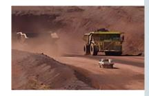
Large dump truck used to carry iron ore and dirt (Roy Hill Iron Ore Project, Australia)
