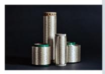
Thread made from recycled cellulose at Circ
