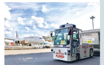
Self-driving towing tractor used in the airport Proof of Concept (PoC) test
