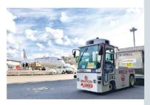
Self-driving towing tractor used in the airport Proof of Concept (PoC) test
